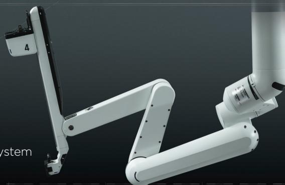
The *da Vinci Xi* Surgical System combines the functionality of a boom-mounted system with the flexibility of a mobile platform. This hybrid architecture enables placement of the surgical cart at any position around the patient while allowing four-quadrant anatomical access.
